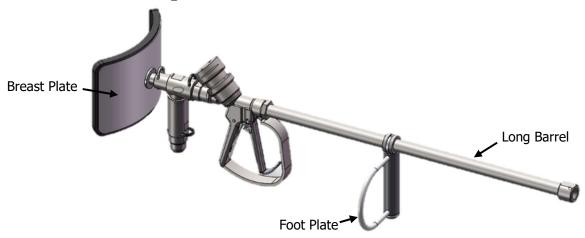
The HPE Standard Cleaning tool is the Cleaning tool that HPE recommends. This Cleaning tool can be used in both standing and sitting positions. The breast plate is used in a standing position and improves jetting control. When the Cleaning tool is used in a sitting position, the foot plate prevents the operator's foot from slipping from the foot rest and injuring the operator's legs. The long barrel assists in preventing accidental body injuries to the operator.
